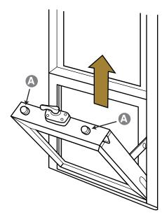
To allow easy cleaning, your window has been fitted with a tilt action.
