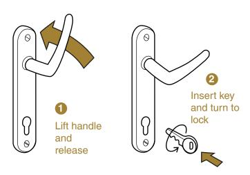
2 Allow the handle to return to the horizontal position. **To deadlock**, turn the key one full turn towards the edge of the door. This will secure all the bolts. In this condition the handle cannot be pushed down. Remove the key and place in a safe location.
