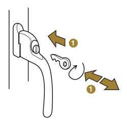
2 . . .then release the catch by depressing the button, and turning the handle.
