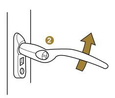
To close the window - fully close the window, turn the handle and lock using the key.
